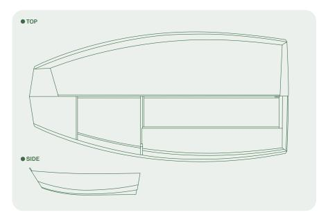
Longitudinal Buoyancy chambers provide floatation where its needed most providing level floatation in the event of swamping
